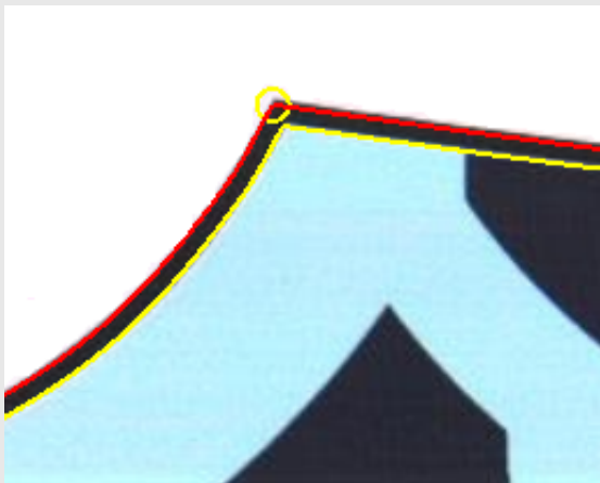
Automatic border detection in printed fabrics. Red: detected contour lines, Yellow: cut-lines, Circle; detected corner
