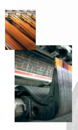
The PDS end out detector detects missing ends during carpet manufacturing. All ends are inspected at any loom speed. The PDS system has been designed for Axminster
